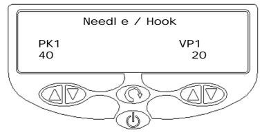
Fig 4.3 Screen for Needle or Hook selected
