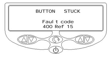
Fig 4.10 Screen for recoverable fault display
