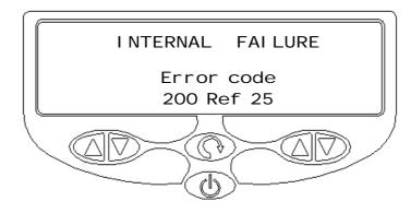
Fig 4.11 Screen for critical error display
