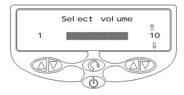
Fig 4.6 Screen for Alarm volume selection
