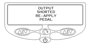
Fig 4.8 Screen for shorting of a non-grasping electrode
